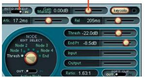
When AUTO MAKEUP is IN, the compressor automatically chooses an appropriate makeup gain for you. This is based on your dynamics contour. You can still use the 'manual' gain makeup control in this case. It merely adds to the makeup gain automatically applied. When you first set the AUTO MAKEUP to IN, the compressor adjusts your makeup gain parameter so that the volume does not suddenly jump up. This is hearing (and speaker) protection!
